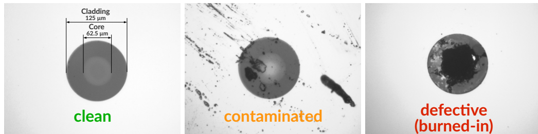
Figure 1: End-faces of optical fiber connector, viewed through fiber microscope
